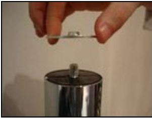
Figure 1. When fitting the washer to the leg bolt make sure the burr on the washer is facing upward away from the leg top.
